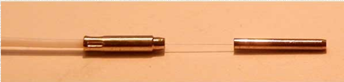
Figure 2b: Dual ferrule pigtail assembly: Front ferrule for optical coupling attachment, Rear ferrule for solder attachment to package wall
