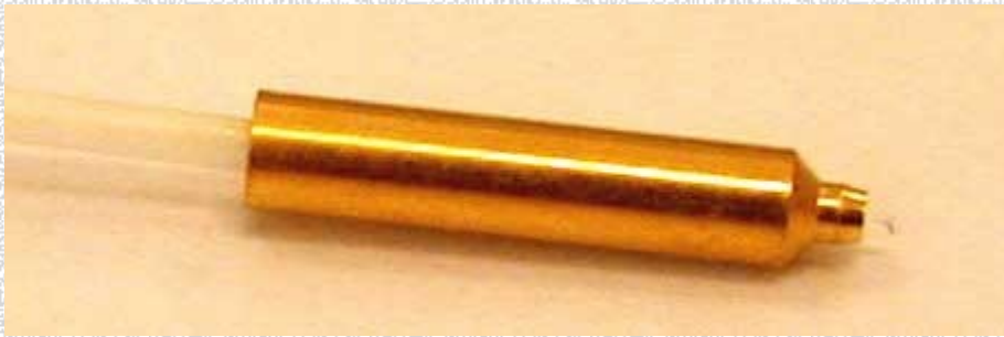
Figure 2a: Ferrule impact mounted to optical fiber. 2.0 mm Kovar ferrule impacted on 8j APC bare fiber with a 0.5 mm protrusion.
